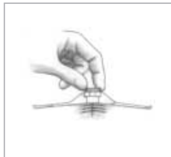
3. To adjust tension, lift capstan.
