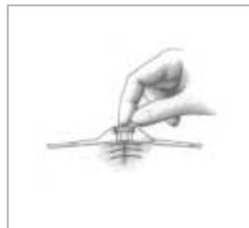
5. To lock, press capstan down into bridge.
