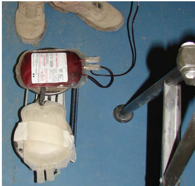
Blood trip scale made from a balance beam scale with improvised counterweight
